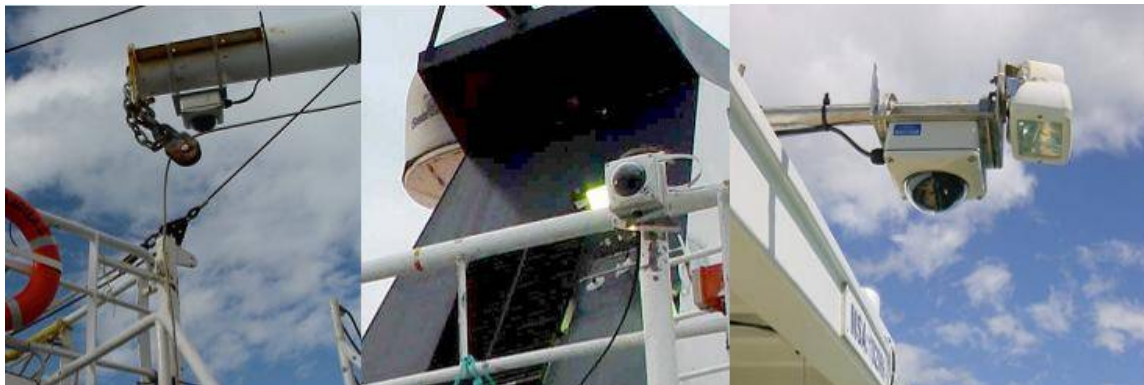
Figure I.2 CCTV camera installations on three different fishing vessels. Each camera has a mounting bracket and stainless steel mounting straps.
