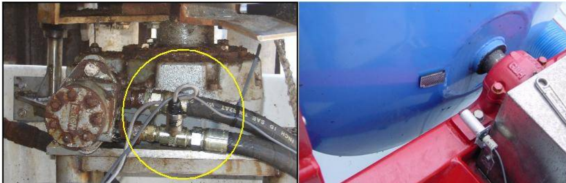
Figure I.5. A hydraulic pressure sensor installed on the supply line of a vessel line hauler (left). Drum rotation sensor (right) mounted on pelagic longline vessel, showing optical sensor and reflective surface.
